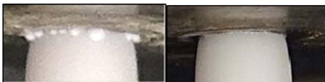
Photo: Comparison of die buildup after 30 minutes without PPA (left) and with 1260 ppm of Kynar® 705 polymer.
